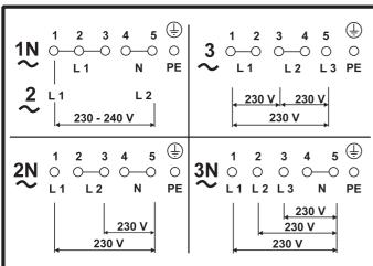
Caution: Incorrect connection results in the total destruction of the power electronics.
